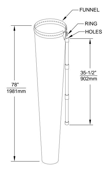
THE MODEL 9010 / 9011 SHOWER TEST KITS GUIDE THE WATER TO A FLOOR DRAIN OR CONTAINMENT BUCKET.
